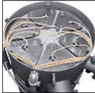
Coil heaters being used to heat up the oil for vacuum generation.
