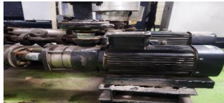
After- installed one 160M-2 type, shakti make, 10 HP IE3 Class one motor with energy efficient pump against two IE1 motors
