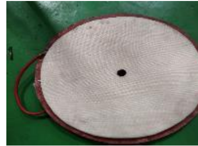
After- Now We developed design for induction heater and installed 16 KW induction heater by removing 24KW triangular all heater. We save 4 kwh per hour
