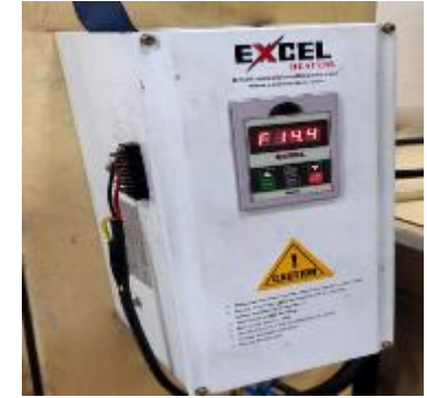
After- Now We developed design for induction heater and installed 16 KW induction heater by removing 24KW triangular all heater. We save 4 kwh per hour
